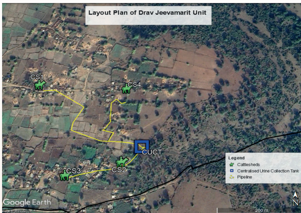
Photo 1: A screenshot of geotagged data on cattlesheds and other resources. This can be used to plan Centralised Jeevamrut units in any region
