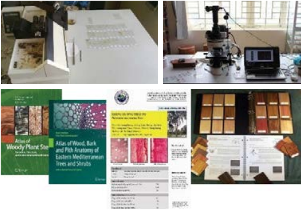
Figure 30: Macroscopic and microscopic features of wood are described using microscope and compared with the database for identification.
