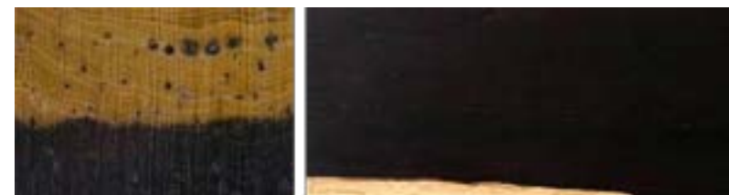
Figure 51: Transverse surface (left) and tangential surface (right) of African blackwood
