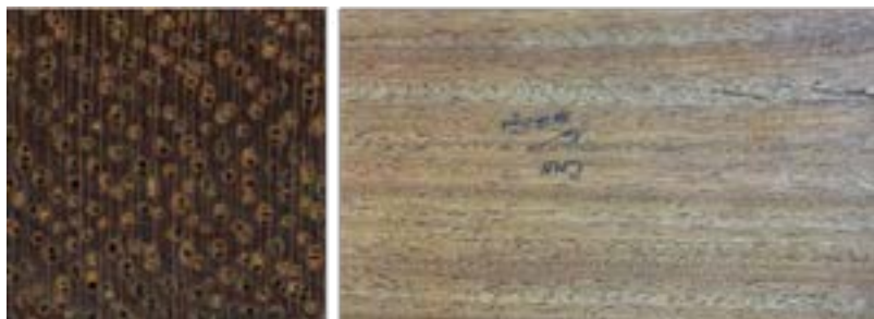
Figure 53: Transverse surface (left) and tangential surface (right) of Okan
