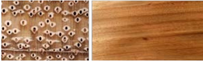
Figure 56: Transverse surface (left) and tangential surface (right) of Bomanga
