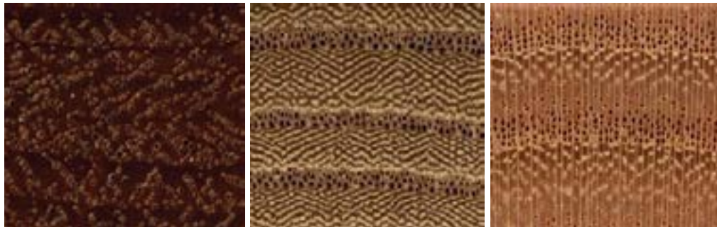
Pores in diagonal and/or radial pattern (Eucalytus marginata)
