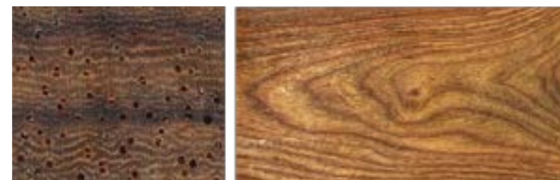
Figure 48: Transverse surface (left) and tangential surface (right) of Ven (Kosso wood) (Source: Internet)
