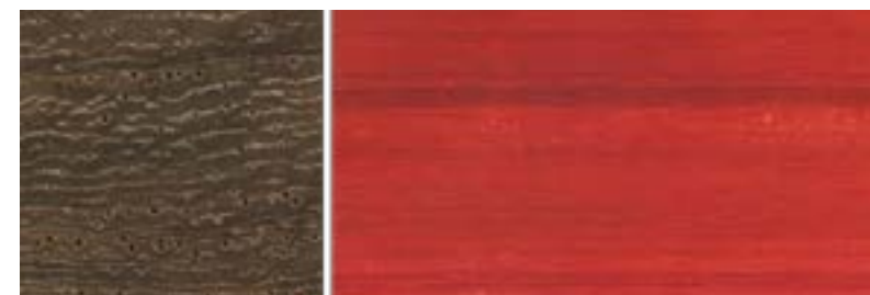
Figure 49: Transverse surface (left) and tangential surface (right) of African Padauk (Padouk)
