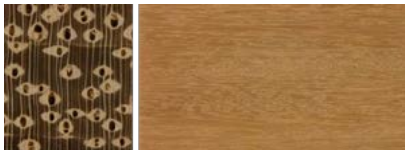
Figure 54: Transverse surface (left) and tangential surface (right) of Doussie
